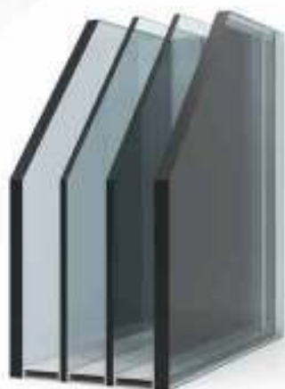
4 glasses, safety glass inside and outside 33.1+4+4+33.1
